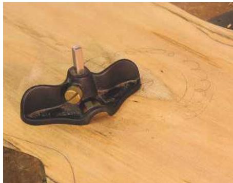
▲ Pic.5 Phil used a hand router to remove the waste, which created a tight fit for the rosette
